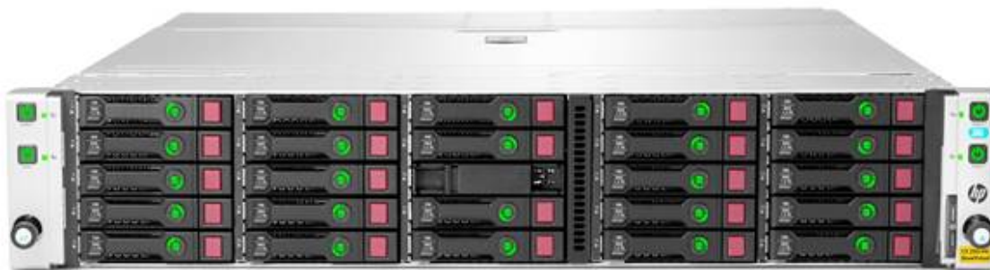
Chassis, front view with 24 drives
