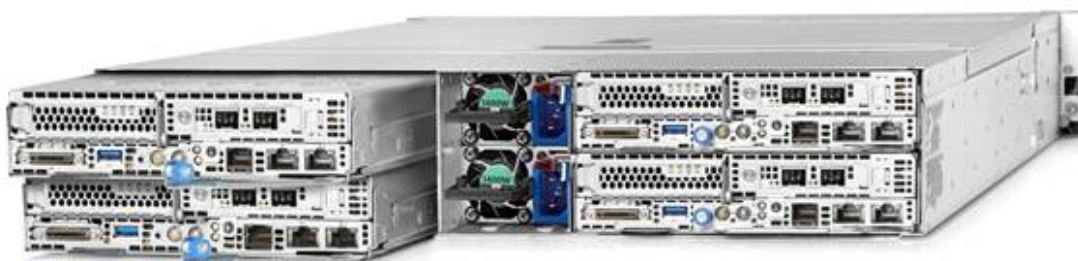
Chassis, back view with 4 nodes
