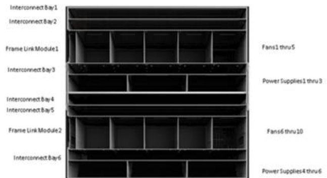
HPE Synergy 12000 Frame - Rear View
