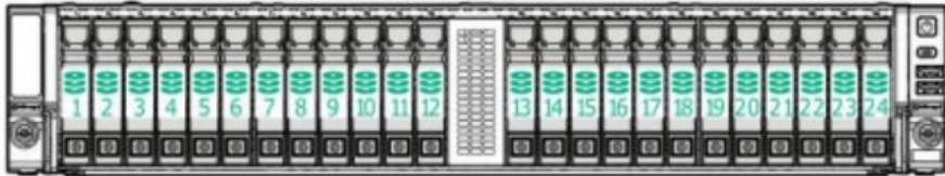
24LFF hot-plug front drive numbering
