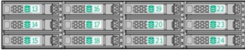
24LFF hot-plug front drive numbering
